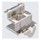
End clamp for fastening photovoltaic modules on support profiles of free-standing systems. Lockable pre-fastening of the module frames on the support profile. Suitable for slot width 10 mm. Lockable fastening of the PV module with Torx 30 wrench.
